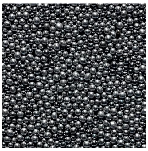
The Ervin technology for stainless steel abrasives is the most advanced worldwide. AMACAST is produced in Tecumseh, USA, using a process developed in the aerospace defence sector, unique in the abrasives industry. This, combined with the knowledge of the stainless team in Sprockhövel, Germany, makes AMACAST the highest quality austenitic stainless shot.
