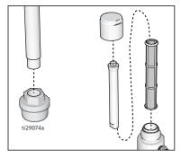
5. Fill throat packing nut with TSO to prevent premature packing wear. Do this each time you spray.
