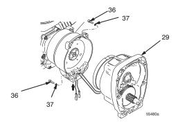
Place pinion assembly (29) on bench with rotor side up.  Remove four screws (28) and lock washers (24). Install two screws in threaded holes (E) in rotor. Alternately tighten screws until rotor comes off.
