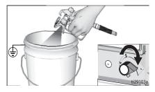
Inspect fittings for leaks. Do not stop leaks with your hand or a rag! If leaks occur, turn sprayer OFF immediately. Perform **Pressure Relief Procedure** steps 1-3, page 8. Tighten leaky fittings. Repeat **Startup** procedure steps 1-5. If no leaks, continue to trigger gun until system is thoroughly flushed. Proceed to step 6.
