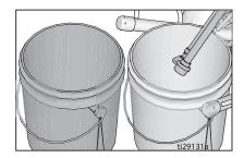
10. Turn prime valve down DRAIN position.
