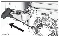
6. After engine starts, move choke to open.
