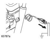
Air and fluid hoses: Use only electrically conductive hoses with a maximum of 500 ft. (150 m) combined hose length to ensure grounding continuity. Check electrical resistance of hoses. If total resistance to ground exceeds 29 megohms, replace hose immediately.
