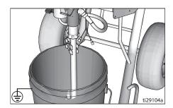
14. Trigger gun again into flushing fluid pail until material appears.
