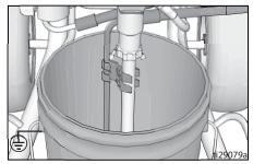
Turn prime valve down to DRAIN position. Turn pressure control counterclockwise to lowest pressure.
