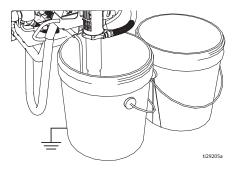
Turn prime valve down to DRAIN position. Turn pressure control counterclockwise to lowest pressure.
