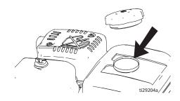
Check hydraulic oil level. Add only Hydraulic Oil, ISO Grade 46, 169236 (5 gallon/18.9 liter) or 207428 (1 gallon/3.8 liter). Hydraulic tank capacity is 1.25 gallon (4.75 liters).
