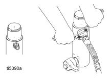
2. Install hose to spray gun and tighten securely.
