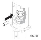
3. Fill packing nut with Packing Seal Fluid.
