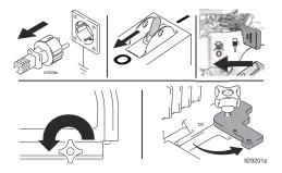
2 Lift belt guard. Remove belt. Tilt engine/motor and remove engine/motor.
