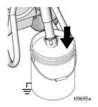
Trigger gun again into flushing fluid pail until paint appears.
