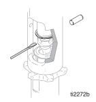
5. Loosen jam nut. Unscrew pump.
