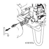
**To ground sprayer:** Attach sprayer grounding clamp to earth ground.
