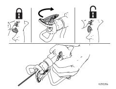
Engage trigger lock. Return tip to original position. Disengage trigger lock and continue spraying.
