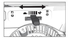
5. Set hydraulic pump valve ON (hydraulic motor is now active).
