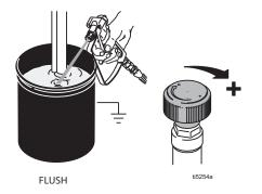
Inspect for leaks. If leaks occur, turn sprayer OFF immediately. Perform Pressure Relief Procedure, page 15. Tighten leaky fittings. Repeat Startup procedure steps 2-8. If no leaks, continue to trigger gun until system is thoroughly flushed. 10. Place siphon tube in paint pail.
