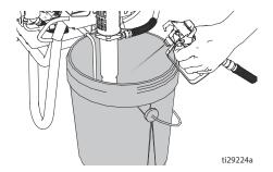
While continuing to trigger gun, turn prime valve down. Then release gun trigger. Allow flushing fluid to circulate until fluid comes out of drain tube clear.
