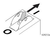
6. Set hydraulic pump valve ON (hydraulic motor is now active).
