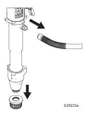
4. Push retaining ring up; push out pin.
