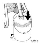
11. Trigger gun again into flushing fluid pail until paint appears.
