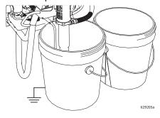
Turn motor switch ON or turn engine ON and start engine. Turn hydraulic pump valve ON. Turn prime valve forward to SPRAY position.
