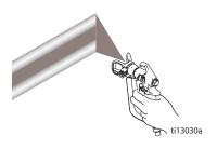
Hold gun perpendicular, 10-12 in. (25-30 cm) from surface. Spray back and forth.
