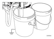
Turn prime valve down. Turn pressure control counterclockwise to lowest pressure.
