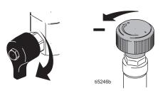
3. Set hydraulic pump valve OFF.
