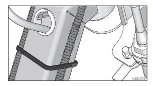
8. Attached laser to desired location on gun arm.
