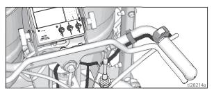
5. Route switch wiring between piston and square tube, and down to battery.
