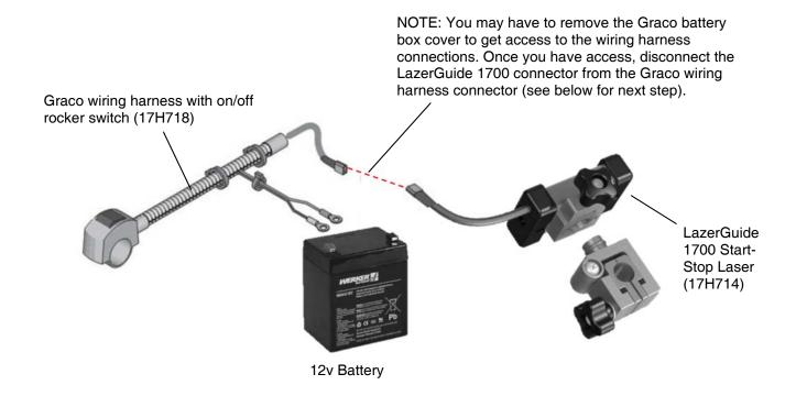
Insert provided Graco "Y" cable adapter (17T537) to the wiring harness as shown. Then connect both the LazerGuide 2000 and LazerGuide 1700 to either one of the two connectors.
