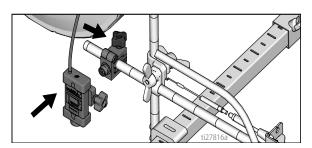
9. Route switch wires down to battery and connect to the (+) and (-) terminals, and route jumper through gun cable hole.
