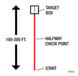
2. At the starting point, make sure your striper frame is true to your reference line by pushing the machine about 10 feet while keeping the spray nozzle over or parallel with the line. Make sure the laser is level, then adjust the laser left-right until it is centered in the target box at the far end.
