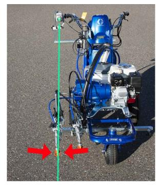
4. Position spray nozzle directly over reference line and maneuver machine left-right until laser is centered in target box at the far end. Make sure spray nozzle is centered over line.
