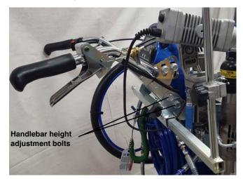
2. Slide new bracket (5) over loosened bolts and securely retighten bolts.
