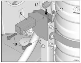
**NOTE:** LazerGuide 3000 Kit installation for LineLazer 250 systems is shown for mounting on existing Pressure Bead System (right bracket). When no Pressurized Bead System is present, order right bead tank bracket 16T697, bolt 111194 (2x) and nut 101566 (2x).
