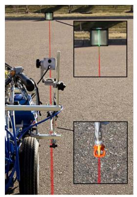
5. Walk towards target box while keeping the laser centered in the target box at the far end. Look only at the target NOT at the spray nozzle. Stop at halfway point and check the position of the spray nozzle relative to the line.
