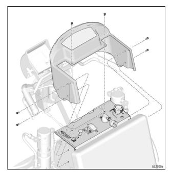
2. Remove circuit board cover with 5/16 nut driver.
