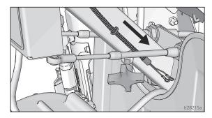
6. Route jumper between piston and square tube, and down to gun cable hole.
