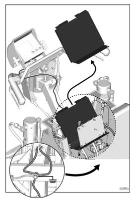
3. Install blue wire tap to the only RED wire having a bullet connector. This is necessary so the battery does not drain over night. For better access, you can remove the key switch.
