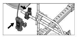
6. Connect the switch leads to the laser wire harness.
