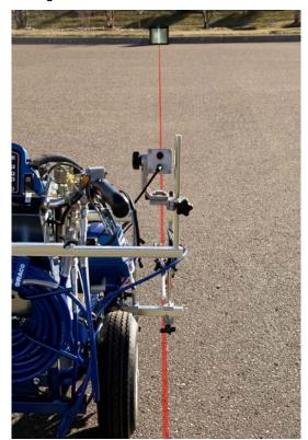
3. Tilt laser downward and swing **spray gun left or right** until it is in line with the laser. Adjust laser back to upward position.
