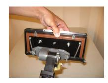
8. The wingnuts should be tightened snuggly by hand, but no tools need to be used to provide a secure connection.
