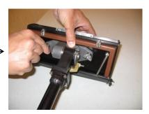
9. The hose is then connected by inserting the quick disconnect pilot fitting of the hose into the grip end of the handle.
