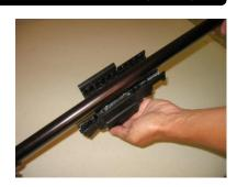
12. The box slide controller should securely snap in place over the shape of the handle and can either be locked into place or allowed to slide freely by adjusting the locking nut on the top side.
