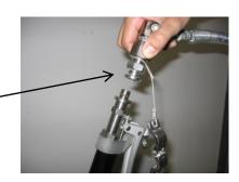
10. Secure by hand tightening the clamp nut.
