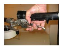
Start compound flow by fully squeezing the valve lever
