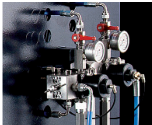
New dosing unit with valves
